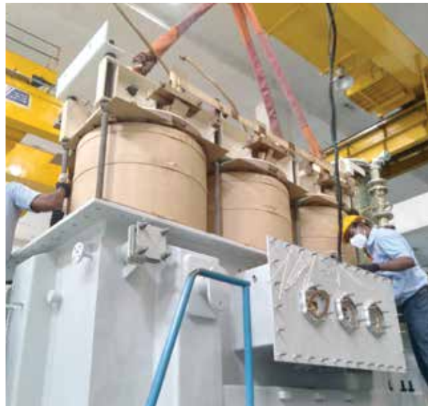
A snapshot of two of the Toshiba transformers being manufactured, which recently underwent a Factory Acceptance Test via Skype.
